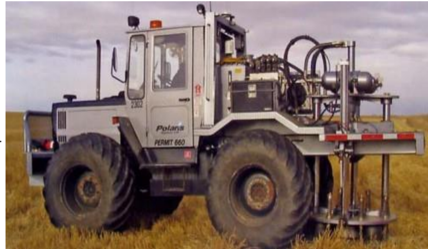
Polaris 860 Seismic Tractor : One of lightest impact seismic source equipment available
